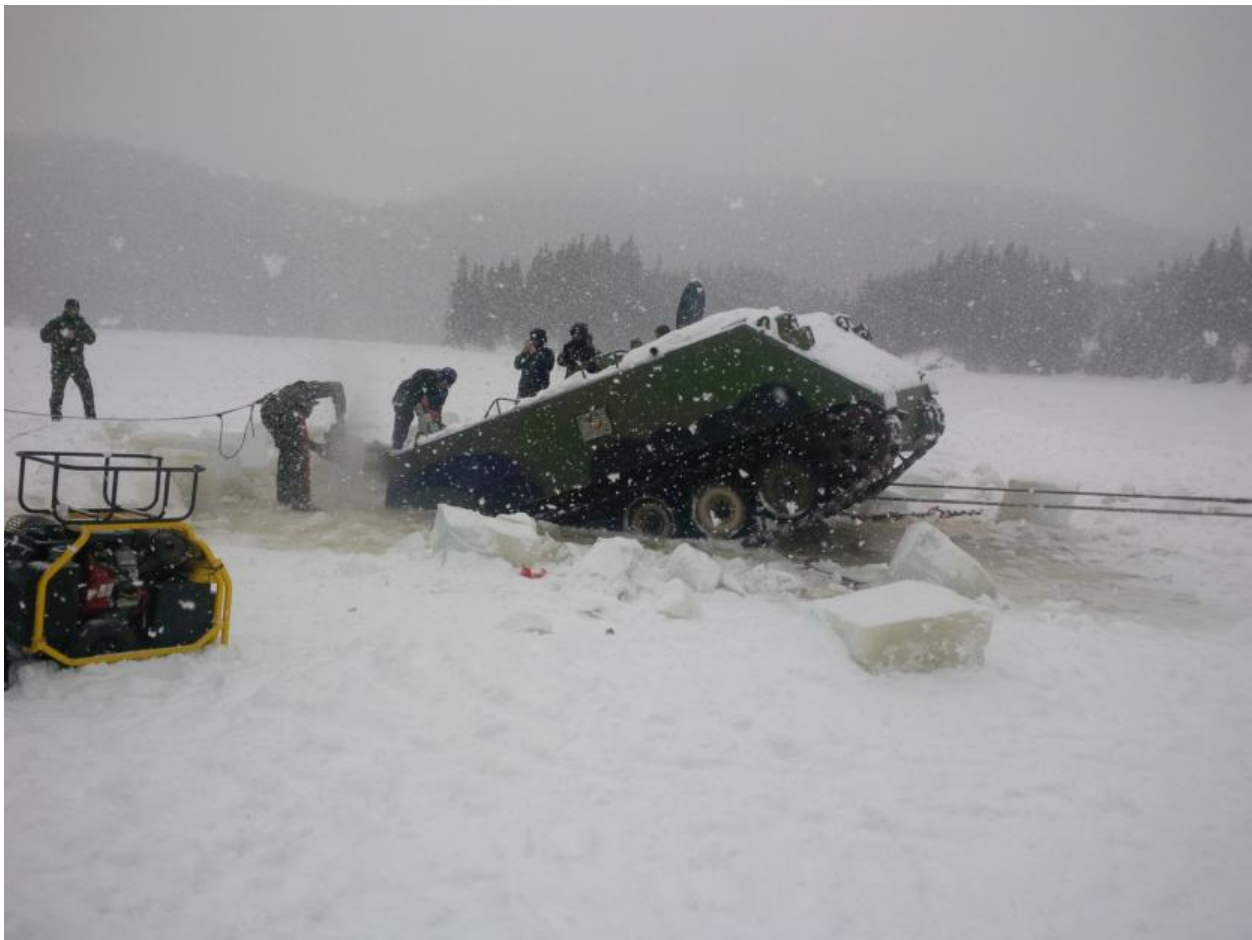
2 CER Dive Team cutting an APC out of the ice.
