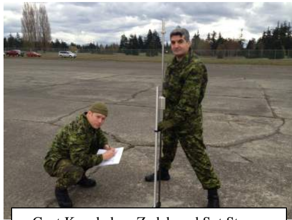
Capt Kouchekan-Zadeh and Sgt Stacey from 8 Wg Trenton, using a Dynamic Cone Penetrometer (DCP) to determine soil strength during the course in Comox.
