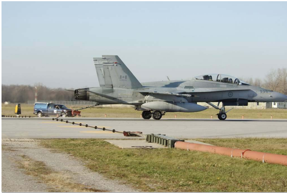
Installation Certification of an AAS at 8 Wg Trenton.
