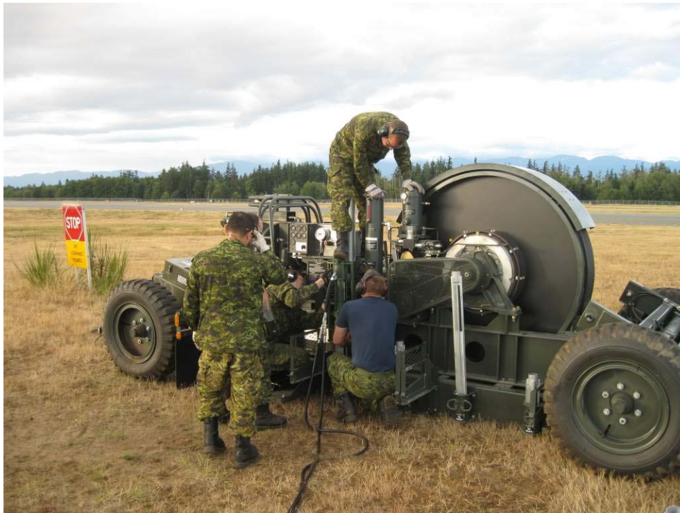
RM Techs installing body stakes on a Mobile Aircraft Arrestor System at CFB Comox. Pers in Photo: MCpl Pollock (86 ASU AAS Tech), Pte Kiley (86 ASU AAS Tech) and 3 x Comox pers (RM Techs) Photographer: Sgt Segall
