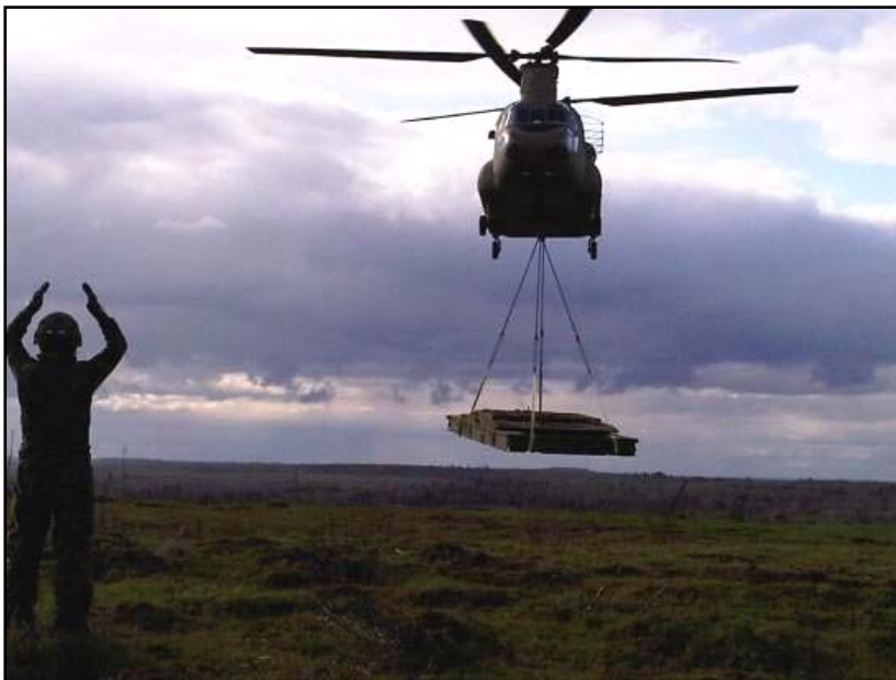
MCpl Rivest from 4 ESR marshalling Medium Girder Bridge 5 Bay Single Story load.
