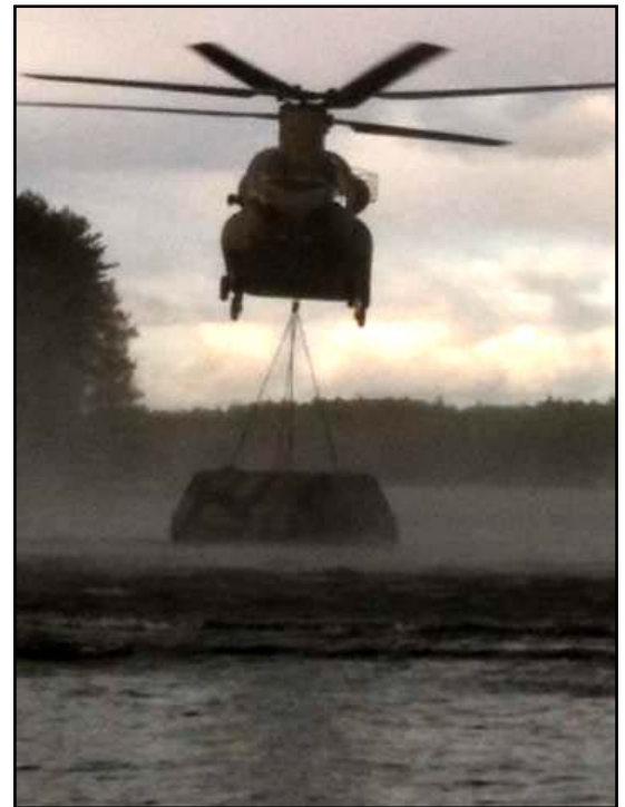
Chinook placing Interior Bay in water at Swan Lake.
