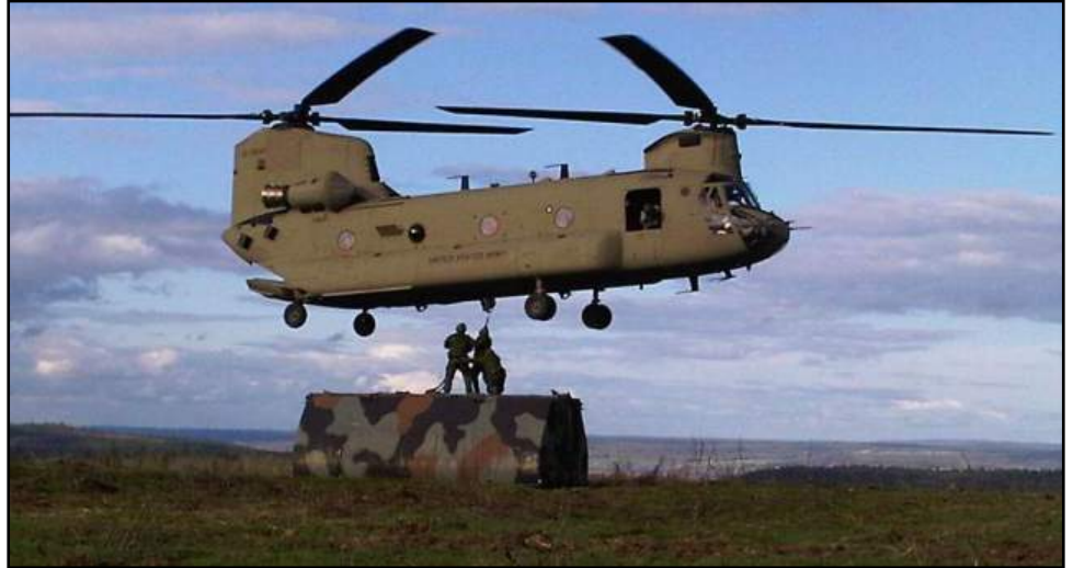
Cpl Pittman, Spr Sturge and Cpl Hicknell (2 RCR) hooking up a MR Interior Bay to the Chinook.
