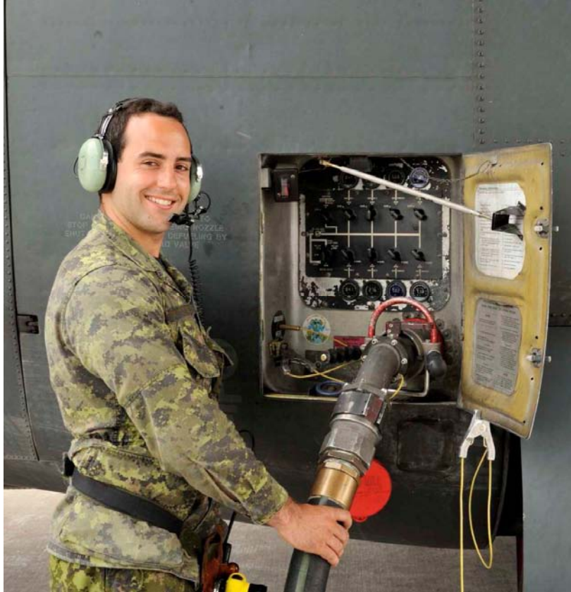
8 Wing personnel fills the Legacy Herc with semi-synthetic jet fuel using 50/50 Camelina bio-jet with F-34 fuel types.
